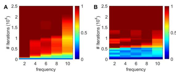
**Figure 2:** Convergence of the amplitude for each frequency during the training process. (A) A neural network is trained to approximate the function  $f(x) = \sum_{k=1}^5 \sin(2kx)/(2k)$ . The color represents amplitude values with the maximum amplitude for each frequency normalized to 1. (B) A PINN is used to solve the Poisson equation  $-f_{xx} = \sum_{k=1}^5 2k \sin(2kx)$  with zero boundary conditions.
