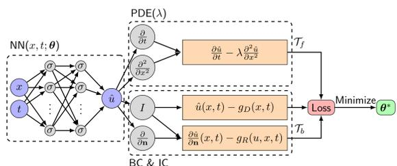
**Figure 1:** Schematic of a PINN for solving the diffusion equation  $\frac{\partial u}{\partial t} = \lambda \frac{\partial^2 u}{\partial x^2}$  with mixed BC  $u(x, t) = g_D(x, t)$  on  $\Gamma_D \subset \partial\Omega$  and  $\frac{\partial u}{\partial n}(x, t) = g_R(u, x, t)$  on  $\Gamma_R \subset \partial\Omega$ .
