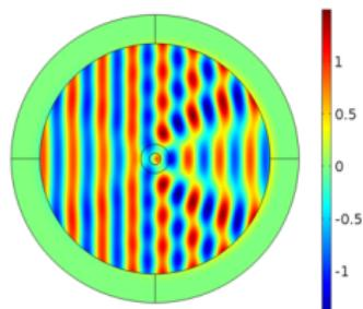
Electric field  $\phi$  with coating
